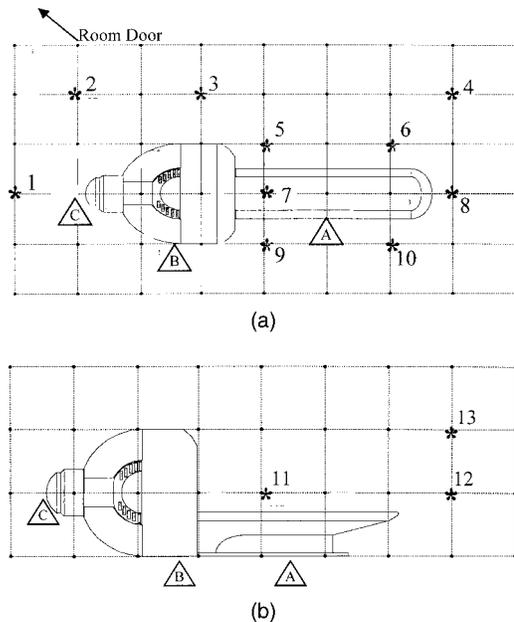
FIG. 4. Scattered radiation measurement locations: Top view (a) and side view (b). Each grid is 90 mm×90 mm. An asterisk and the corresponding number indicate where the measurement was done. The triangle points to the locations of emergency hand wheels: (A) to move the couch out to, (B) to close the shielding door and (C) to close the secondary shutter.
