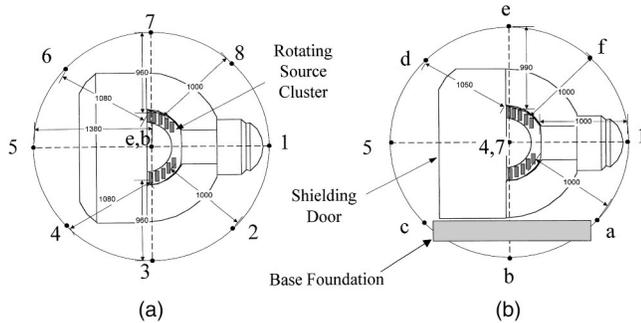
FIG. 3. Leakage radiation measurement locations around the source housing at approximately 1 m from the focal spot: Top view (a) and side view (b).
