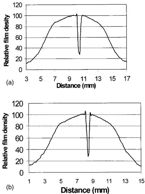
FIG. 7. Mechanical accuracy of the RGS<sub>u</sub>. Pinprick results obtained with the 4 mm collimator. (a) and (b) correspond to the scans in the X and Y directions of the XY plane, respectively.
