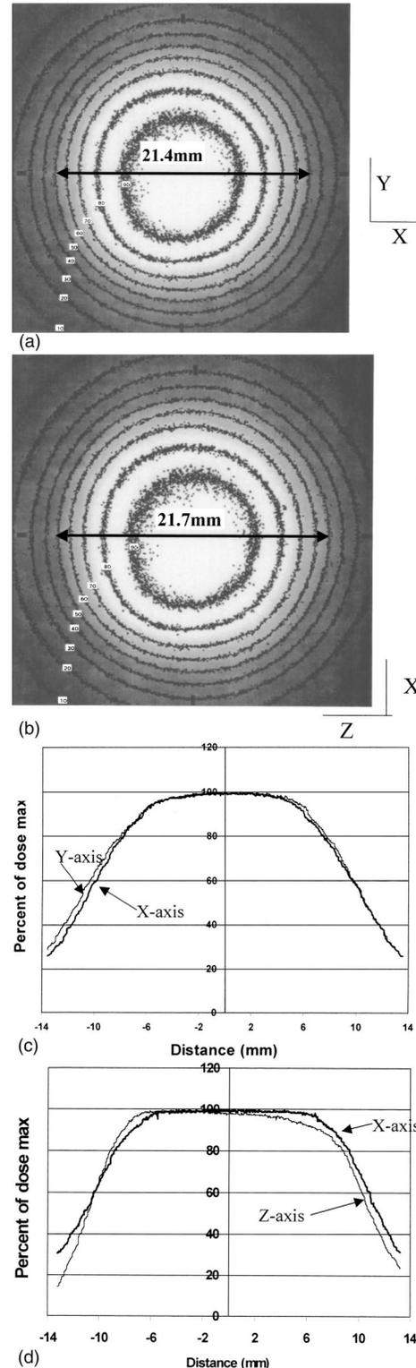
FIG. 6. Dose contours with the 18 mm collimator film exposure on the XY (a) and the XZ (b) planes. (c) The 18 mm collimator profiles in the X and Y axes of the XY plane and (d) in the X and Z axes of the XZ plane.
