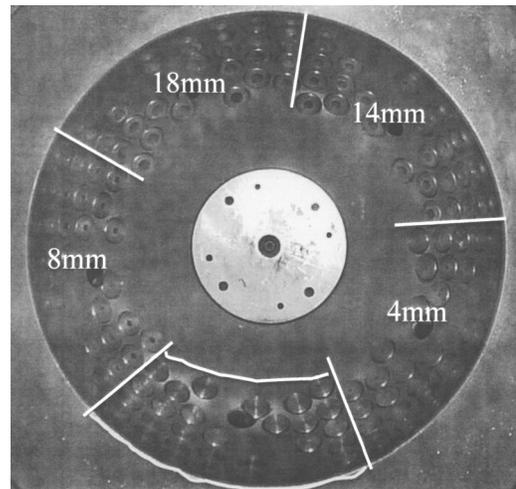
FIG. 2. Secondary collimator body. Five sets of collimators are arranged from the bottom. They are shown clockwise from the bottom, the blocked, 8, 18, 14, and 4 mm collimators.
