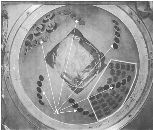
FIG. 1. Primary collimator body. Six arrows indicate the locations of the original source containing cylinder bores, two of which are already plugged. All of them are eventually plugged. The white enclosure in the lower right-hand corner is the new source cluster.
