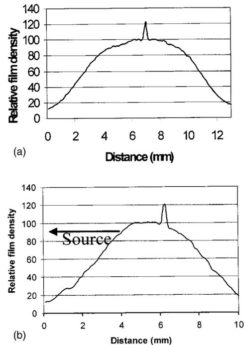
FIG. 8. Pinprick results obtained with the 4 mm collimator. (a) and (b) correspond to the scans in the X and Z directions of the XZ plane, respectively.
